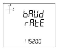
RS-485 communication speed of the device can be set to one of the following options:
