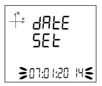
The date of the device's RTC module can be set in days, months and years.
