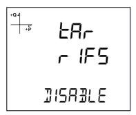
Press the SET button. If you change Disable option to Enable with UP/DOWN buttons, tariff function of the device will be activated. Press the SET button to confirm your selection.
