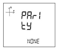
Communication parity of the device can be set as Odd, Even or None.
