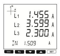
To see the minimum, maximum and demand values of power parameters, first select the relevant screen with "P PF" button.
