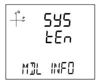
Information about the module that is installed on the device can be displayed under this menu.
