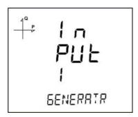
3. Pulse Input: When this option is selected, the device can count the pulses that occur on the input. It can display the pulse count on monitoring screens under "Pulse Cntr C-1" section.
